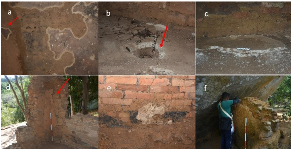
Fig. 3. Location of Sampling a. Dammaruchi Cave wall plaster b. Mahalena floor plaster c. Mahalena floor plaster with two layers d. Buddha Dattha Cave wall plaster e. Korawakgala cave wall plaster f. collecting samples for analysis
